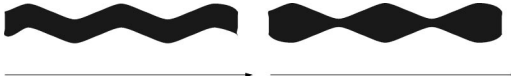
FIG. 7. Sketch of the symmetric (left) and antisymmetric (right) modes of dirt modulation.
